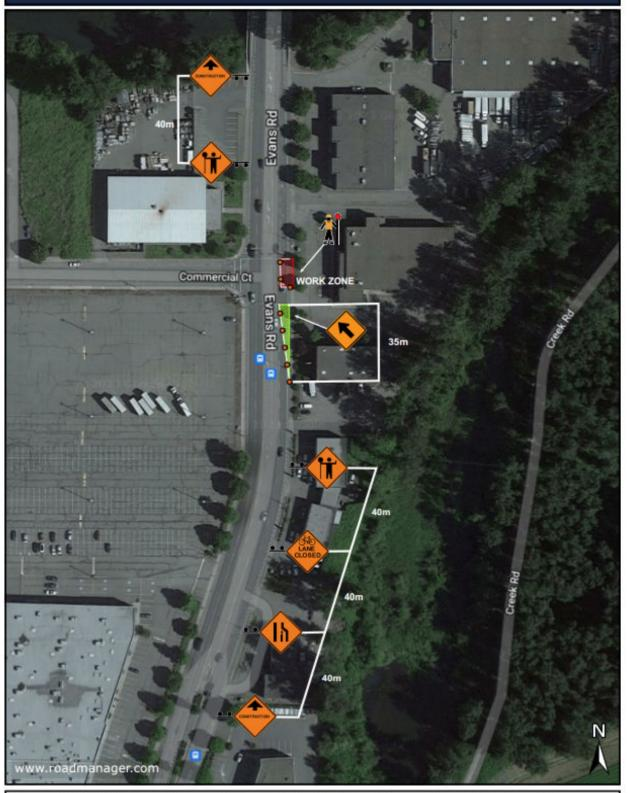
Figure 11.6: Right Lane Closure (Near Side) – Multilane Intersection – Short and Long Duration
